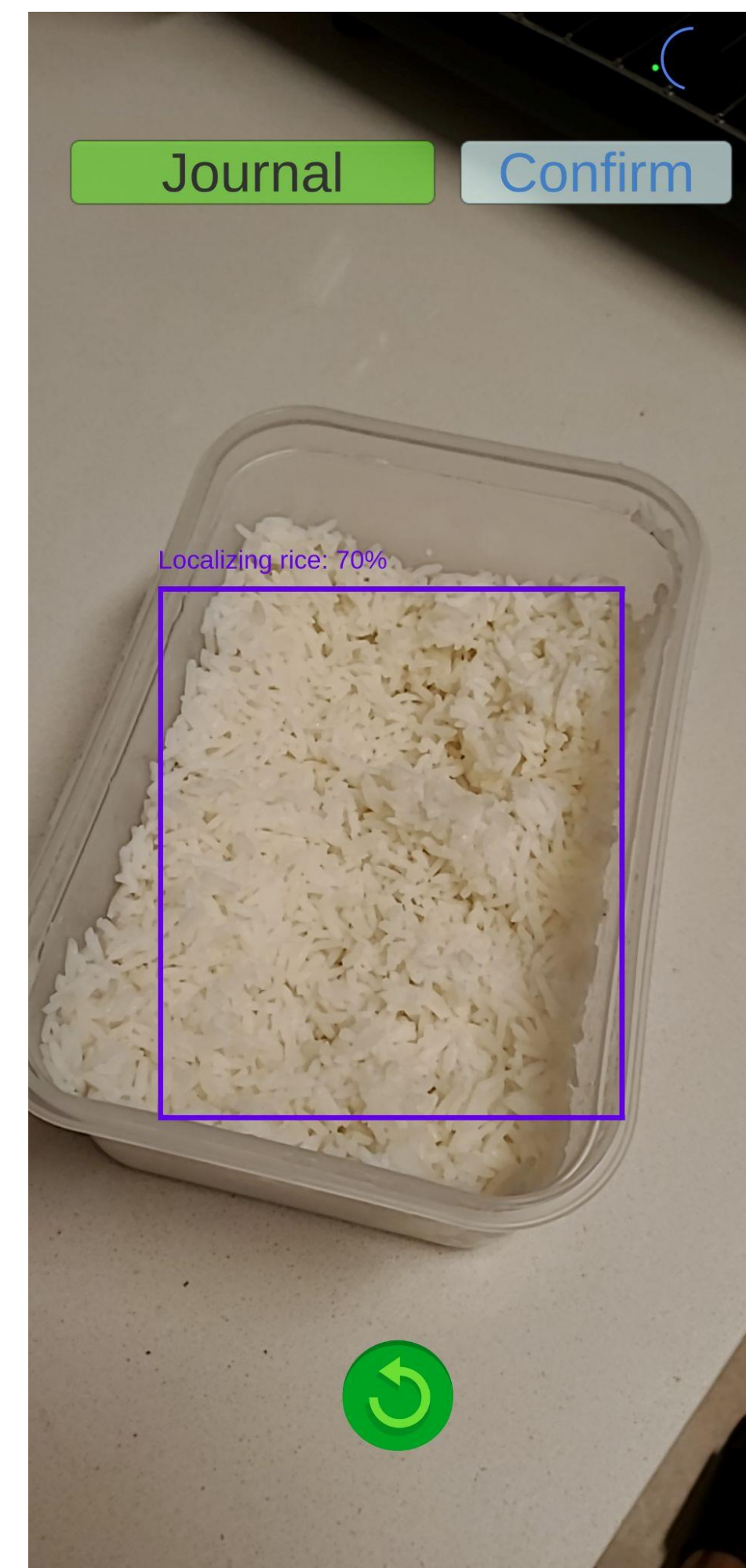
Main screen for computer vision using YOLOv8 object detection using FoodX-251 database
